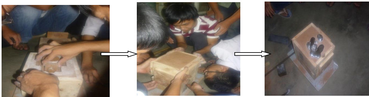
Figure 8: Placing the core, fitting the mould. and pouring melted aluminium
