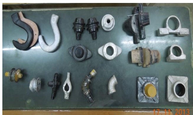
Figure 2: Casting part and their wooden pattern made by students
