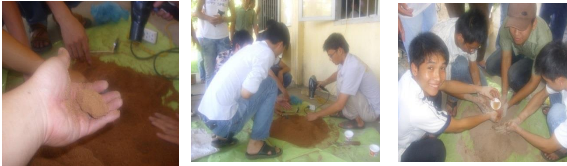
Figure 6: Check the mixture; when the mixture is too wet, it must be dried. When the mixture is too dry, add more water
